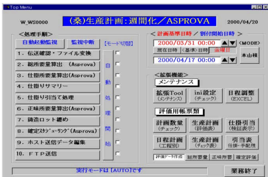
Figure 4: Main menu of production schedule. A range of demands from the production site is reflected. Asprova's processing can be executed automatically using the automation function.
